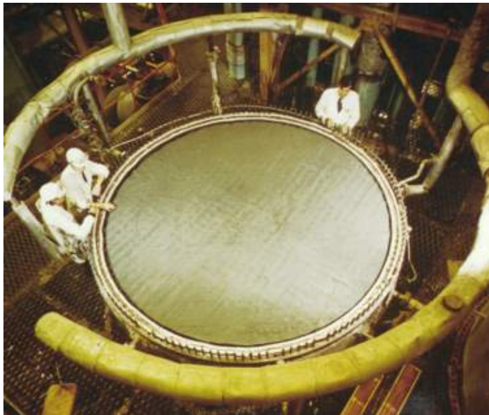
Pt-Rh catalysts used in Ostwald process
