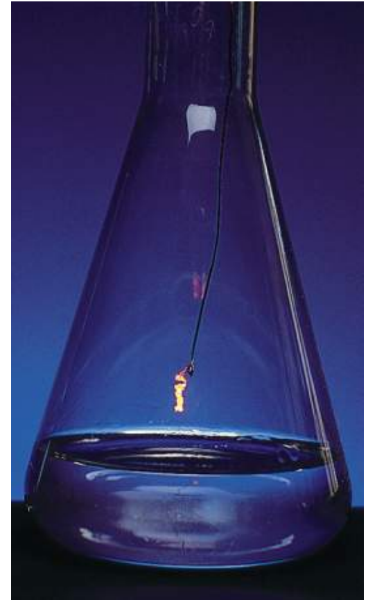
Hot Pt wire over NH 3 solution
